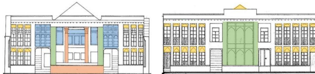
Figures 4 & 5. From the left: General view of the decorations of the western and eastern facades of Mohtasham house, scale 1/100. Bricklaying (yellow), tiling (green), sculpting (red), sash (orsi) and qavarebori (blue). Source: https://farschto.ir .
