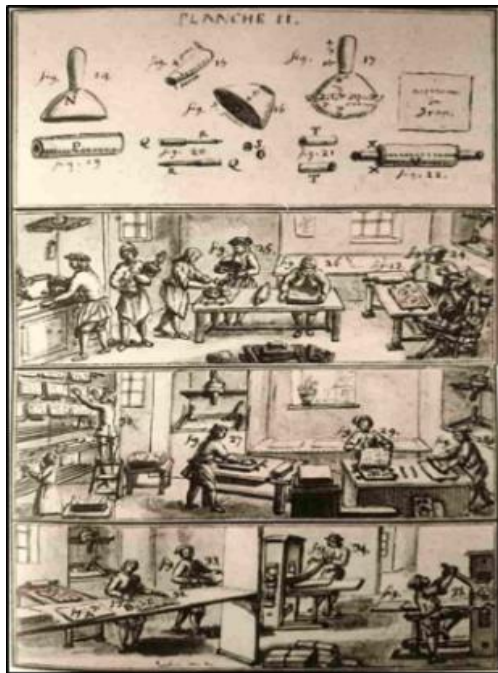
Fig 2. Papillon's drawing of the stages of wallpaper production. 1. Tools needed in the printing process. 2. Mixing the paint, preparing the tool, and using it on the block. 3. Print the sheets, hang them to dry. 4. Dehumidification and arrangement of printed papers. Source: Wisse, 2005, 17.
