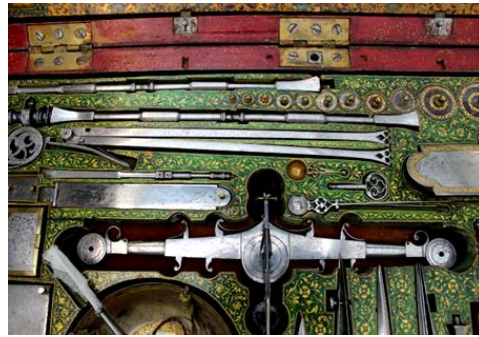
Fig 32. View of the leveling hook and the optimal division of space inside the box. Source: British Museum.
